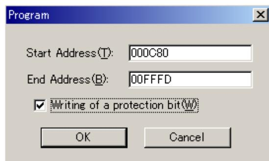
Fig 4.1: Protection functional setting screen
