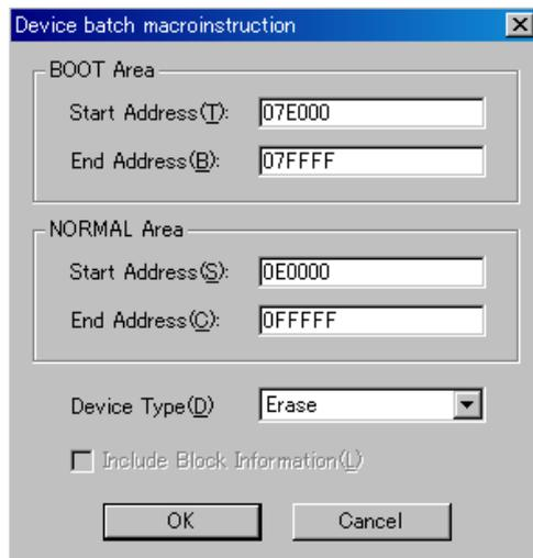
Fig.6.1 Device batch macro command parameter input dialogue
