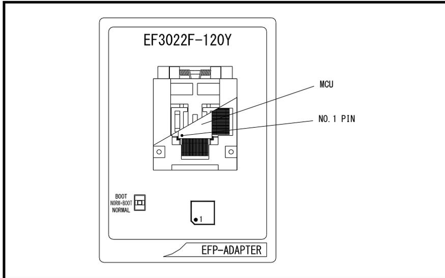
Figure 2.1: Pin Orientation of The socket
