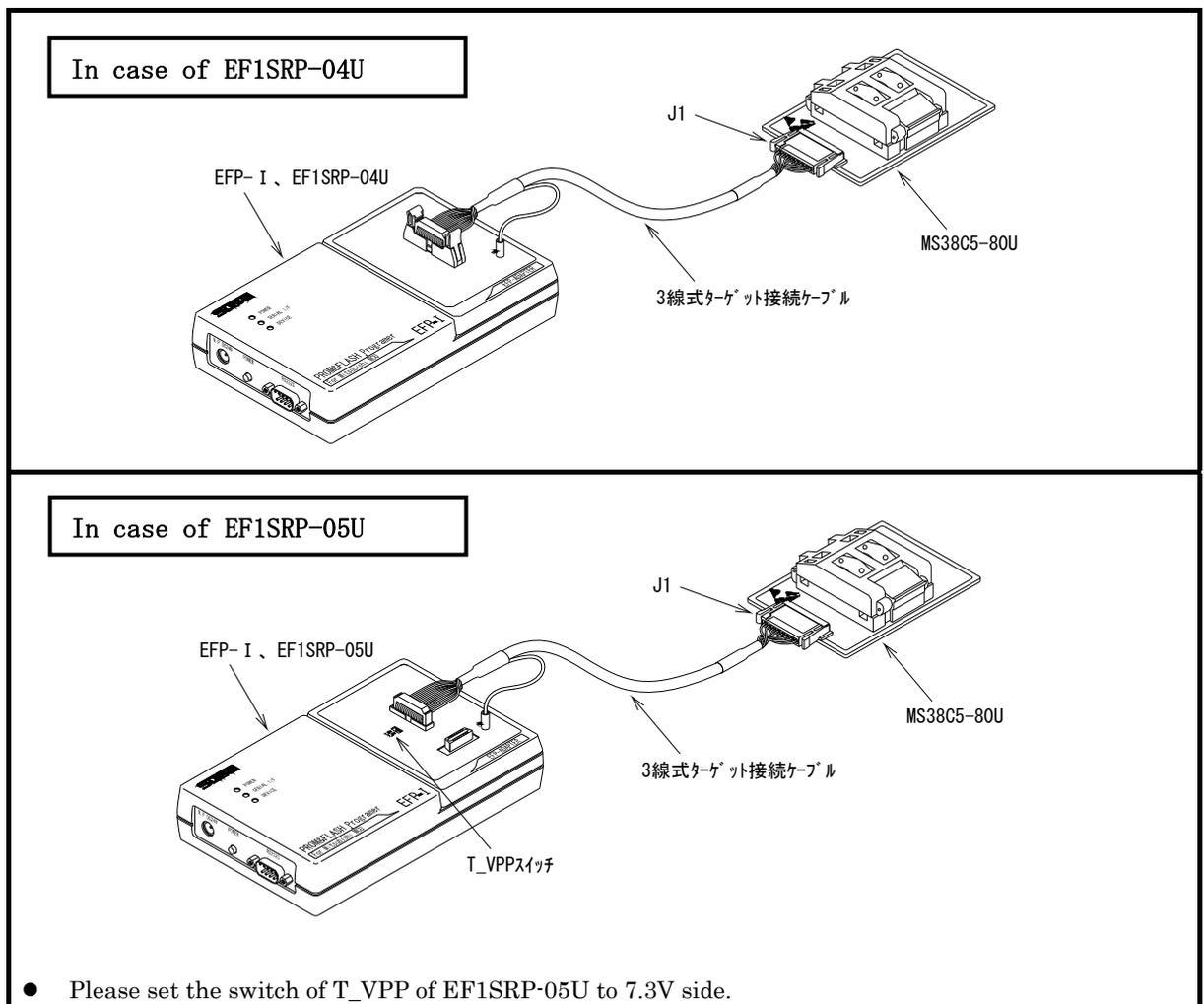
Fig2.1 Connected to EFP-I
