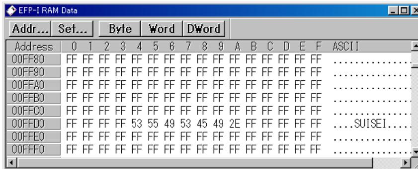
Fig. 7.2 Dump Window (ID Code Setting Data)
